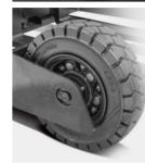
The front wheels are equipped with deep groove rubber tires, with large ground clearance, wear resistance and durability, and good shock absorption effect.
